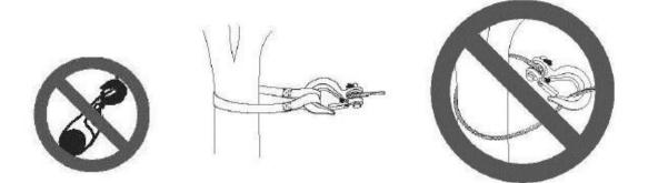
Do not wrap the Rope around the object and hook onto the Rope itself. This can damage the object being pulled, and kink or fray the Rope.
