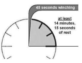
Do not attempt to pull full rated load for more than 20 seconds. Release Power-In switch immediately when winch drum/rope stops. Allow winch to cool and change rigging as needed before continuing pull.
