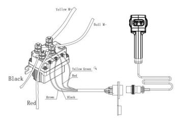
13. Operate the pendant controls briefly to ensure they work properly. If operation is reversed, the power cables may be connected backwards. Correct any such issue before use.
