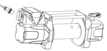
13. Operate the pendant controls briefly to ensure they work properly. If operation is reversed, the power cables may be connected backwards. Correct any such issue before use.
