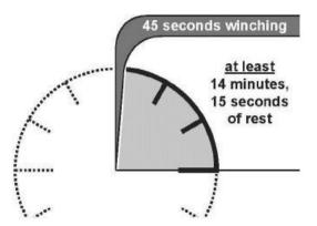
Do not attempt to pull full rated load for more than 20 seconds. Release Power-In switch immediately when winch drum/rope stops. Allow winch to cool and change rigging as needed before continuing pull.
