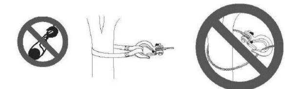
Do not wrap the wire rope around the object and hook onto the wire rope itself. This can damage the object being pulled, and kink or fray the wire rope.
