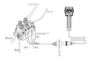
13. Operate the pendant controls briefly to ensure they work properly. If operation is reversed, the power cables may be connected backwards. Correct any such issue before use.
